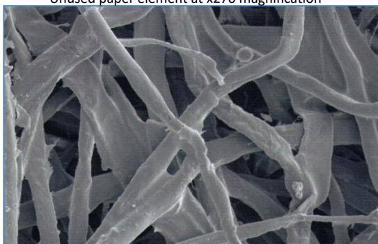
Unused paper element at x270 magnification
