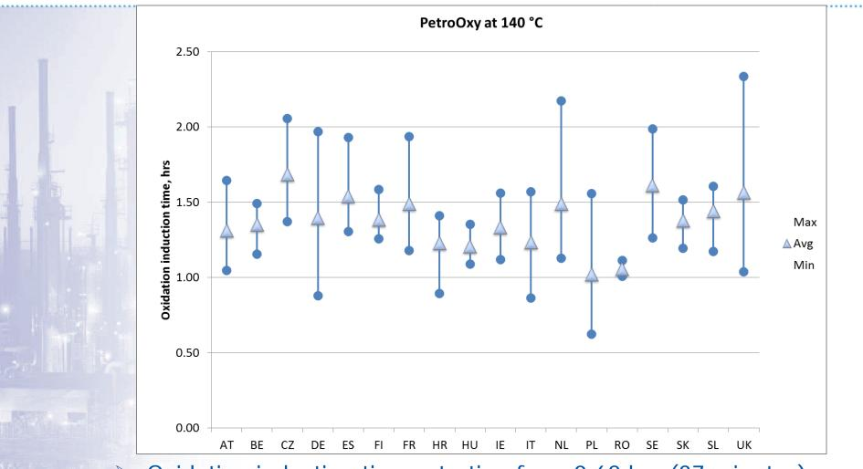
Oxidation induction times starting from 0.62 hrs (37 minutes) observed with PetroOxy at 140° C
