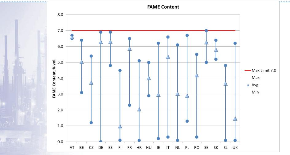
FAME content of all diesel fuels according to EN 590 specification requirements. In some cases diesel fuels without FAME (B0) observed
