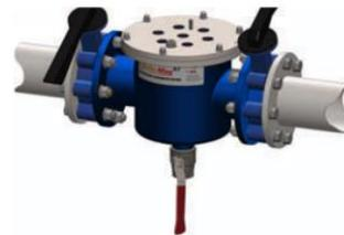
4. Either place a bucket underneath or connect a hose to the 1 1/4" drain valve on the underside of the unit. Remove the drain plug and open the drain valve.
