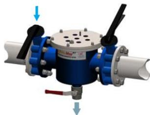
5. Partially open the inlet isolation valve and allow the contents to drain through the drain valve. When the draining water runs clear turn off the inlet isolation valve and allow the remaining contents to drain.
