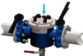
7. Replace the magnetic core and hand tighten the black tricone to retain.
